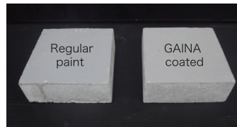
▲Two concrete blocks, with a thickness of 50mm (2 inches), were coated with regular paint and GAINA, respectively.
